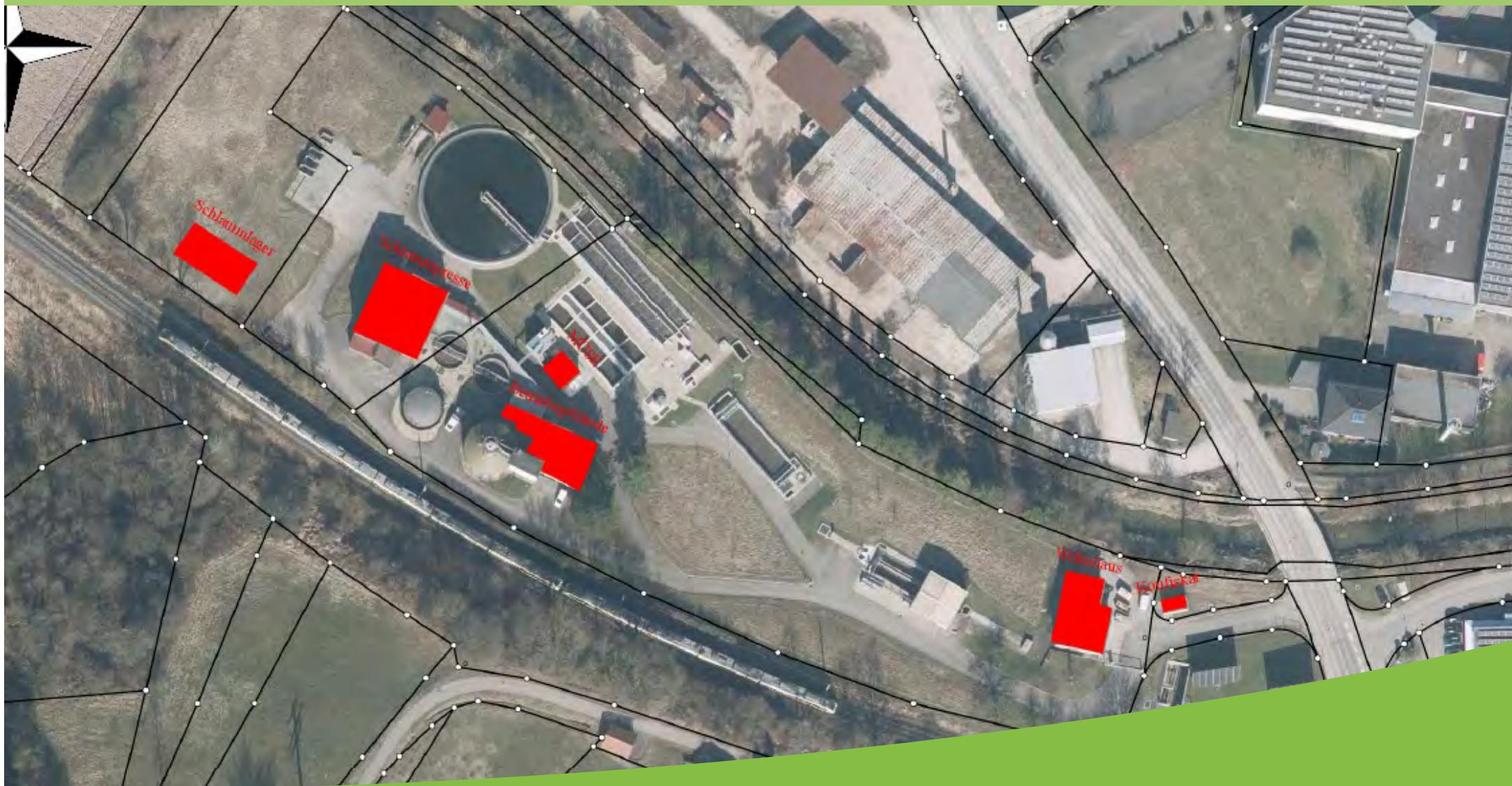
With new solar systems installed on the roofs of the sewage treatment plant, with a combined heat and power plant in which the resulting sewage gas is converted into electricity, and with the existing solar trackers, the sewage treatment plant with its consumption of around 400,000 kWh can be set up in an energy-neutral way.
